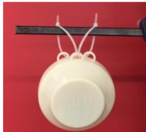
Figure 4. Example of AirU on a hanging mount.
