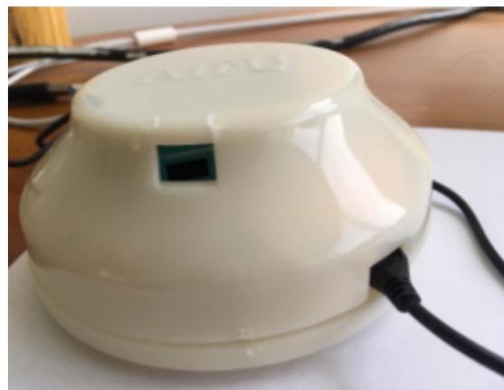
Figure 3. Closed AirU sensor.
